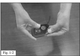
(b) Slide the SmartAccess Remote into the glove and gently adjust the fit by sliding the key glove windows into position (Fig. 1-2).
